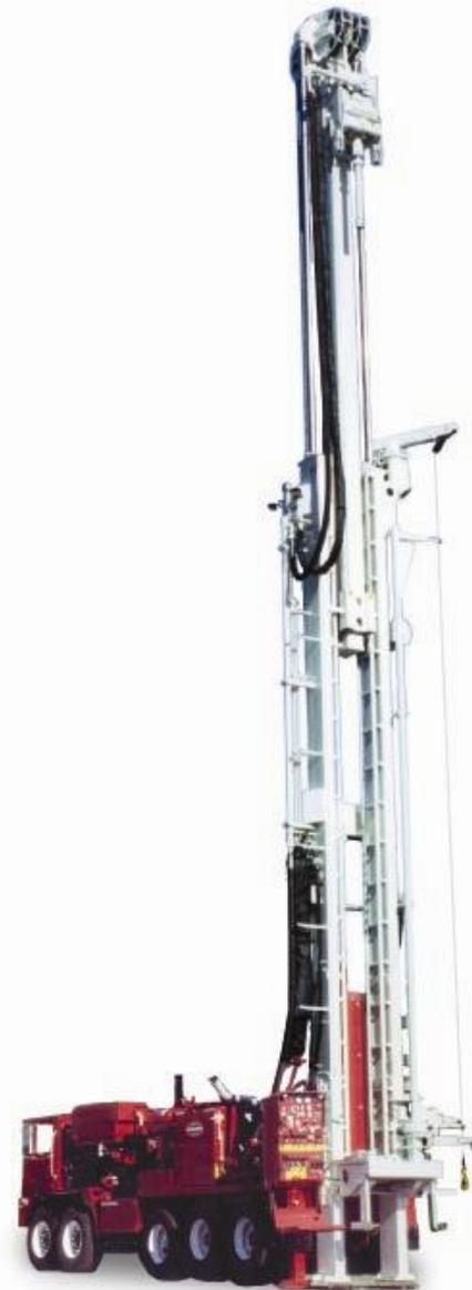
CARRIER MOUNTED RIG EQUIPPED WITH TELEMAST
